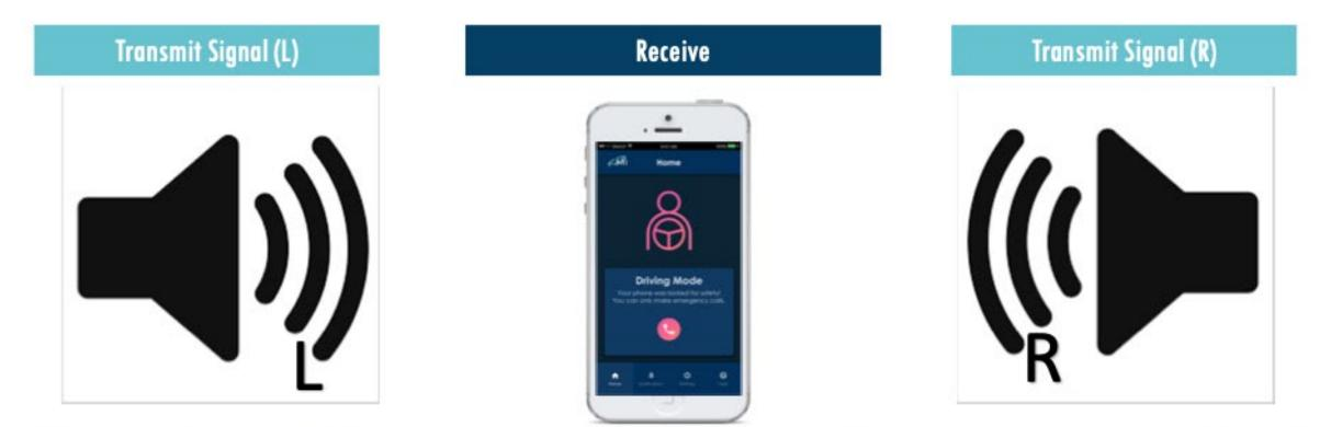
Software algorithms on mobile device receive signal (L) and (R), based on time of flight principle, calculate mobile device location to within +/- 3cm accuracy. This precise location information is passed to fleet integrator's application in order to make mobile device policy decisions as to which work vs. social apps driver can access while mobile device is located in driver's zone and vehicle is moving.
